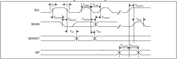
Figure 12. Write Cycle Timing
